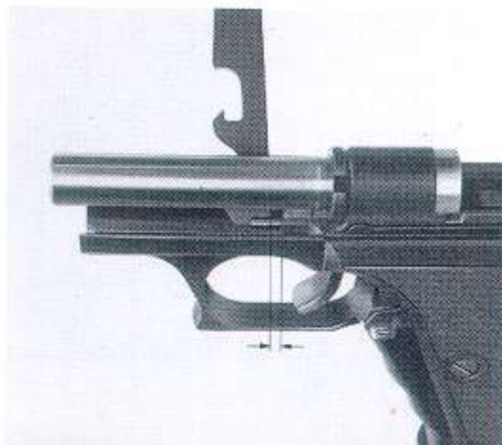
Fig. 19: Check buffer pin protrusion
