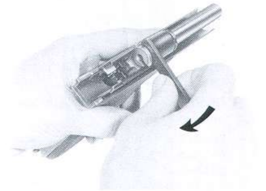
Fig. 14: Pushing the chamber to the rear
