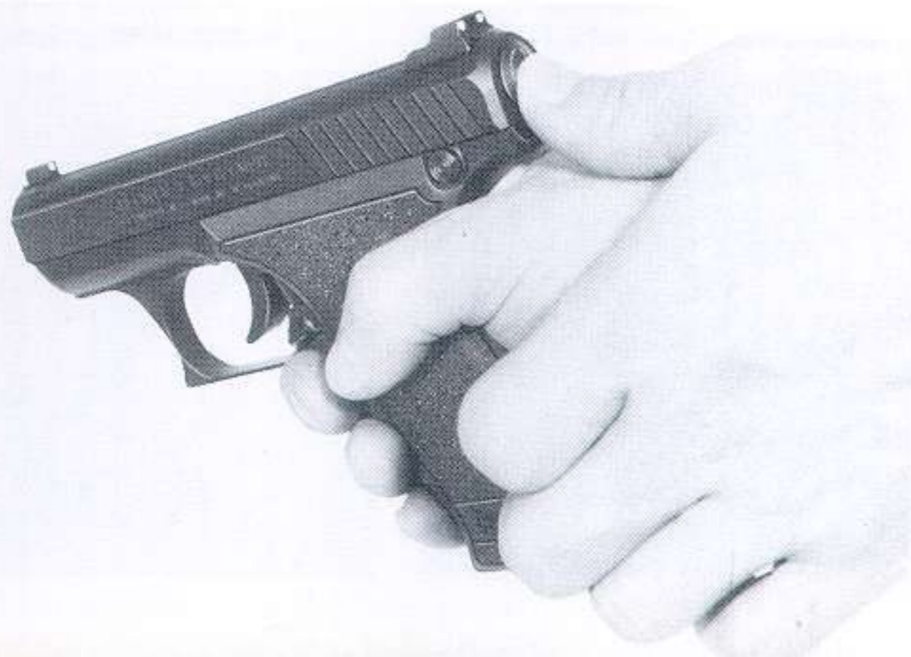
▼ Fig. 17: Press firing pin bushing forward
