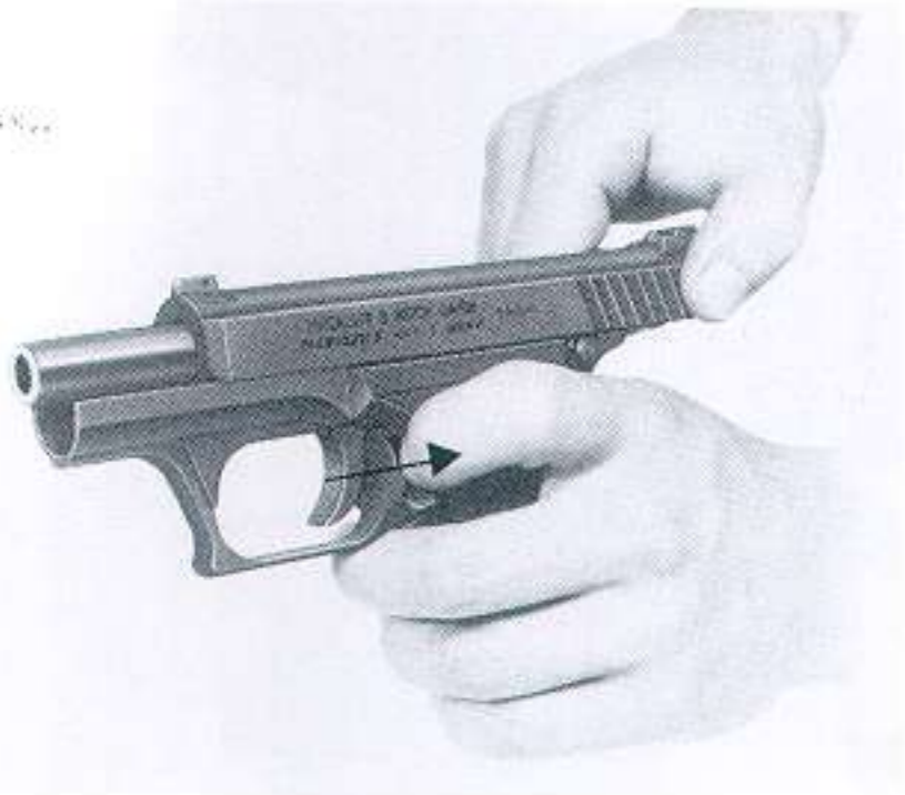
Fig. 6: Press in slide catch lever
