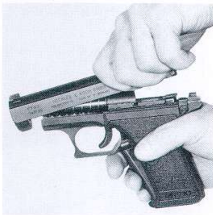
Fig. 9: Place slide on receiver
